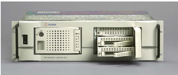
Half- and full-height expansion bays increase capacity.
