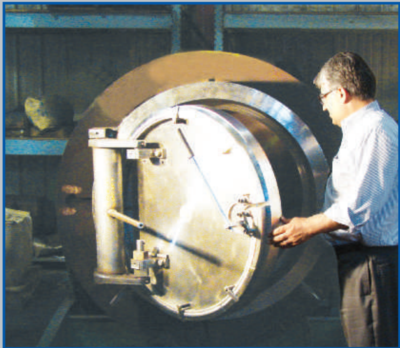
36" CL600 Tool-less™ Closure in Production.
